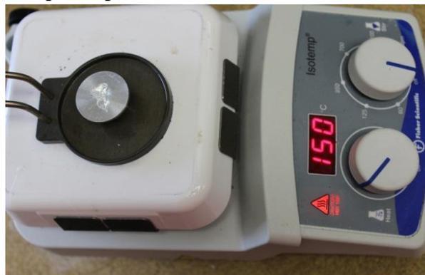
*Figure 4 – Melt wax on the holder to temperature recommended by wax manufacturer*
