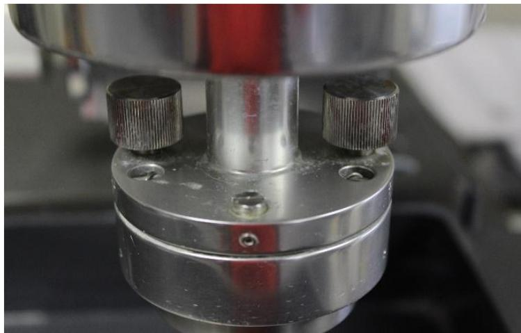
*Figure 6 – Example of leveling thumbscrews on a lap and polishing machine*
