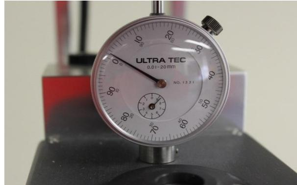
*Figure 7 - Example of controls on a polishing arm and measurement dial for load pressure*
