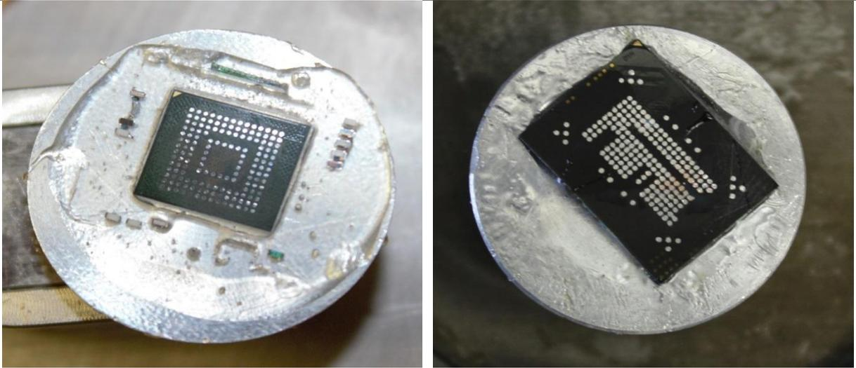
*Figure 9 – Example of circuit board and solder mask removed*
