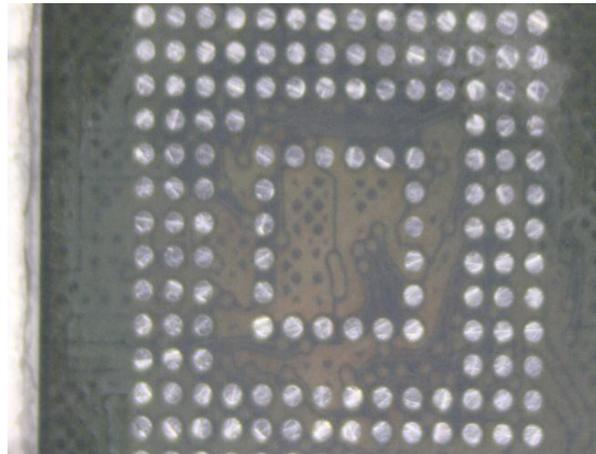
*Figure 10 – Example of BGA package under microscope that was removed by the lap and polish process*
