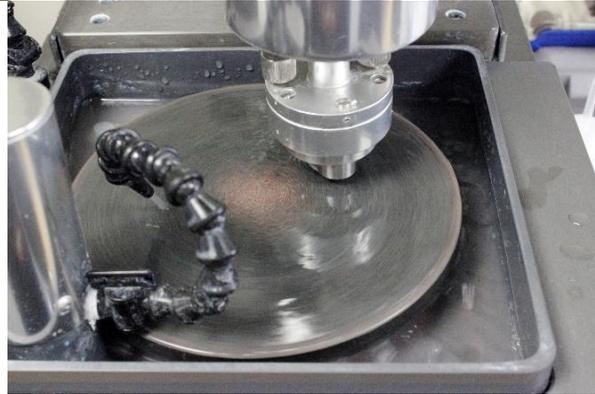
*Figure 8 – Example of polishing wheel powered on and coolant circulating*
