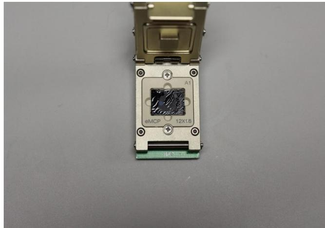
*Figure 11 – Example of NAND flash memory chip that was removed from the circuit board via Lap and Polish Process ready to be read in a chip reader*
