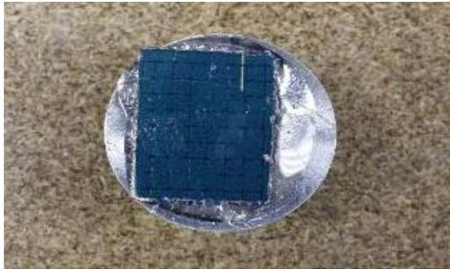
*Figure 3 – NAND flash memory chip with circuit board intact attached to holder*
