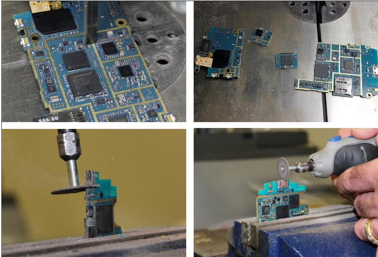
*Figure 2 – Methods for cutting flash memory from a circuit board*
