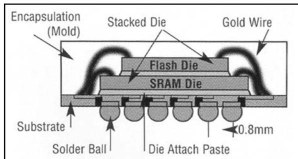
Fig. 2 Chip scale package
