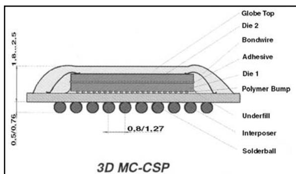
Fig. 3 Schematic of CSP from MPD showing stacked chips
