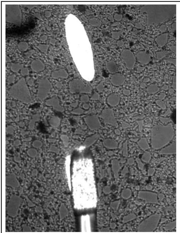
Fig. 6 View of the wedge bond associated with one of two identical power pins. The other was left intentionally unbonded for illustration purposes.
