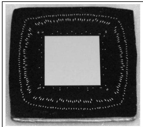
Fig. 7 Polished BGA die in the original package ready for die attach and wire-to-wire bonding in a new package
