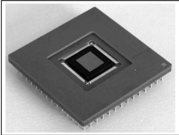
Fig. 5 The sample is die attached with room temp. epoxy to a 132 lead ceramic pin grid array and wire bonded
