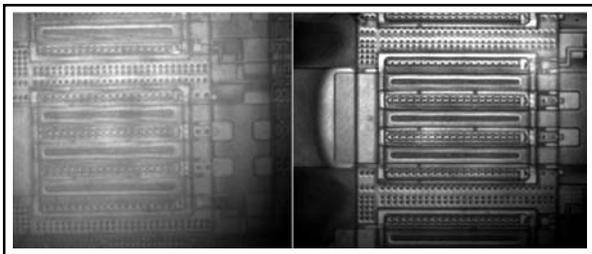
Fig. 8 The finished product with ARC coating on the right and none on the left. (100 $\times$  NIR objective)
