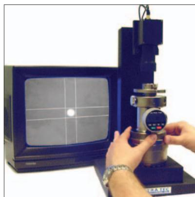
Optical tools such as an ultracollimator allow for increased parallelism of the sample during topside deprocessing.
