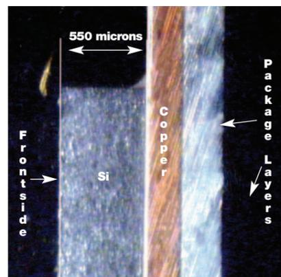
Cross-section of a semiconductor package – annotated to show typical layer types and thicknesses.
