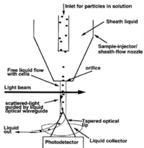
FIG. 1. Sketch of a flow cytometer with the flow-stream-waveguide configuration to collect perpendicular light scatter.
